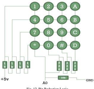
Fig. 12. Pin Reduction Logic
