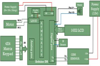
Fig. 11. Hardware Architecture
