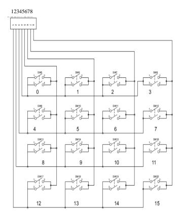
Fig. 8. Keypad Internal Connection
