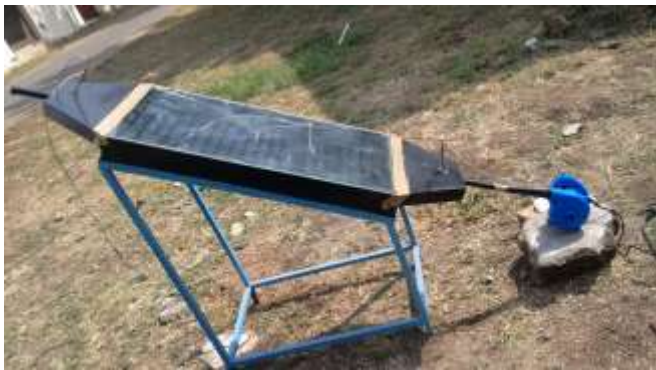
Fig. 2 corrugated black coated Solar flat plate collector
