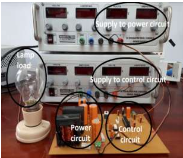
Fig 14. Experimental set up
