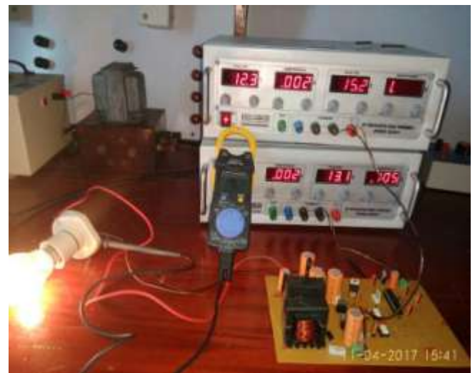
Fig 15. Experimental result showing MPPT operation
