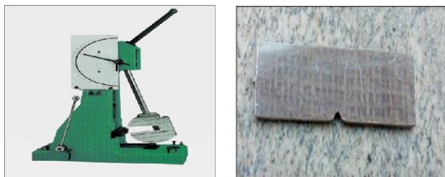
Fig.4: (a) The Izod impact apparatus of capacity of 800N; (b) Tested impact strength sample as per ASTM-D256
