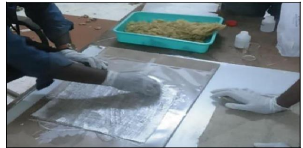
Fig. 1: (a) The first layer glass fiber mat with jute fiber by hand lay-up method;
