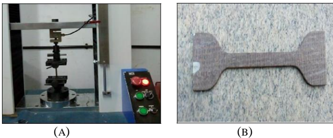
Fig.3: (a) The Universal testing machine of capacity of load 100kN; (b) Tested tensile sample as per ASTM-D638
