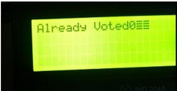
Fig -8: Message on LCD of re-voter
