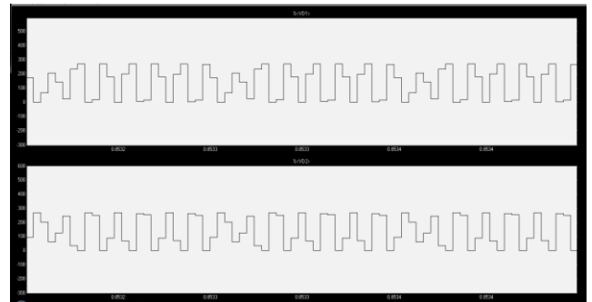
Fig. 5 Waveforms of voltages across D_1 and D_2
