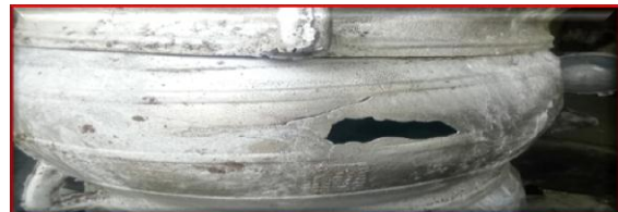
Fig. 2: A pot casting with defect
