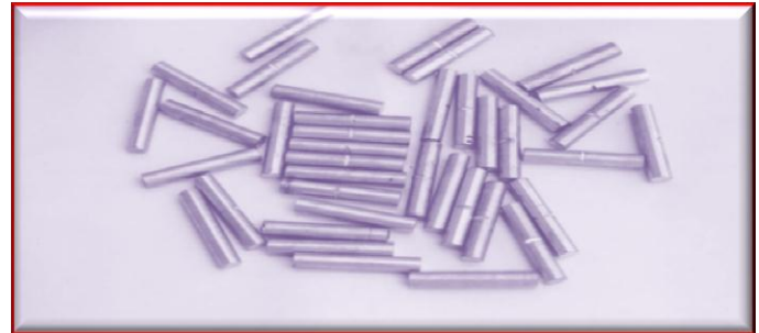
Plate VIII: Some of the produced impact test samples
