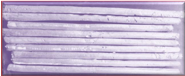
Plate VI: Some of the sand-cast aluminum rods
