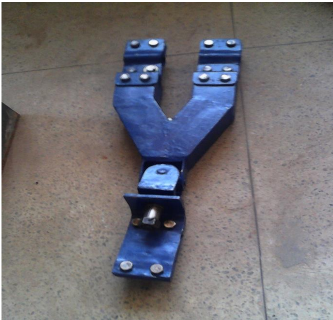
Fig. 8 Fully developed motorcycle trailer hitch
