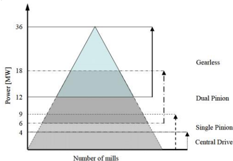
Fig 7.1 Typical mechanical mill configurations [4]
