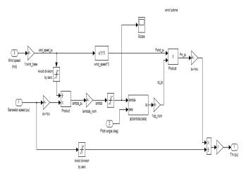
Fig..5 Simulink model of wind turbine
