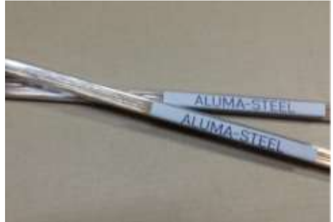
Fig. 2. Shows welding rod- filler rod
