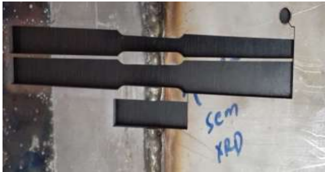
Fig. 5. Samples for SEM and XRD
