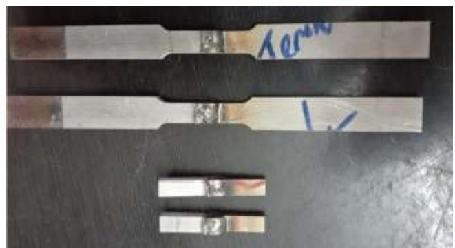
Fig. 3. Tensile and hardness testing samples
