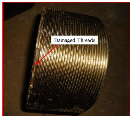
Fig. 1 Damaged threads on thread rolls
