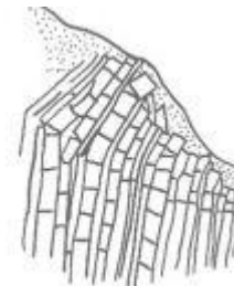
Fig 5. Block Flexural Toppling
