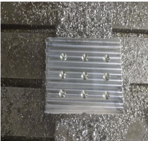
Figure5. Drilling operation on CNC machine
