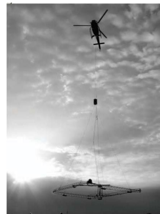
Fig. 7. (a) The SkyTEM system in operation during the spring of 2003 over Sabro, a 40 km 2 survey area west of Aarhus, Denmark. The box between the helicopter and the transmitter lattice contains computers and power supply.
