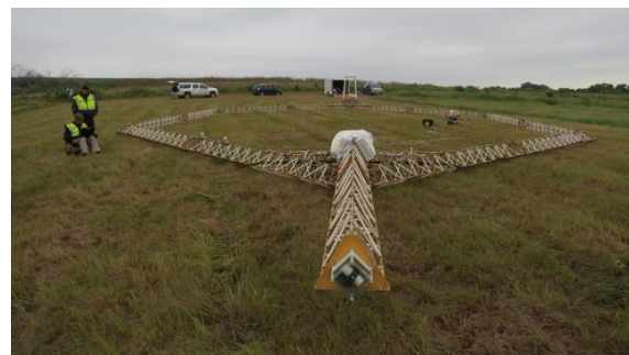
Figure 3 Technicians prepare the SkyTEM rig for aerial mapping.
