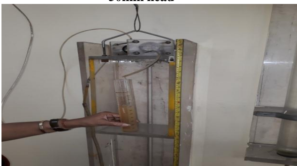
Fig. 14: 2% \text{Na}_2\text{CO}_3 treated/activated CI (ND) soil at 50mm head
