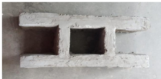
Figure 4: Cross section of papercrete panel
