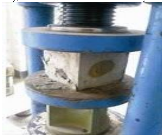
Figure 5: Compression test on concrete cube
