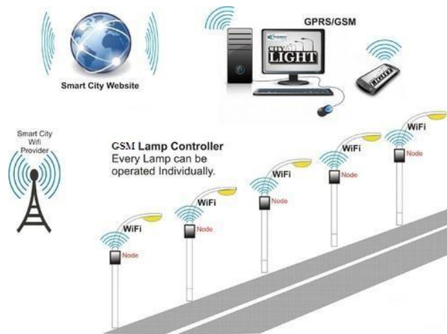
Fig 1. Street light controller with wireless technology
