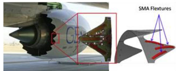
Figure 1 [A] Chevrons with Variable Geometry Chevrons have flight test hardware[21]
