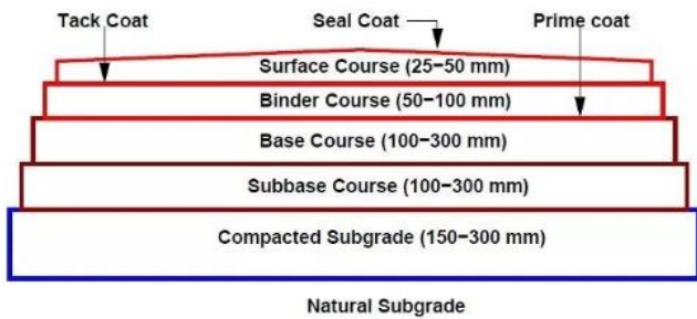
Fig. 1 Typical Cross Section of Flexible Pavement
