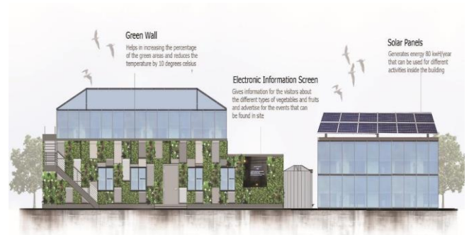
Fig. 19 The main elevation of the green walls, information boards and solar panels
