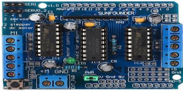
Fig 2.3 - Motor driver L293D
