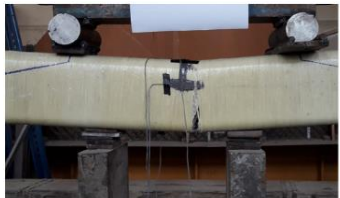
Fig. 5. Tension Failure pattern on bottom flange
