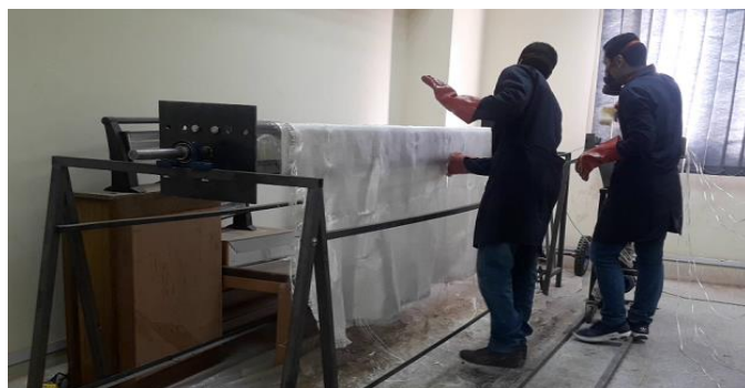
Fig. 2. Stacking the fiber sheet manually (or by hand lay-up technique)
