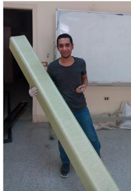
Fig. 3. Final product of GFRP tube
