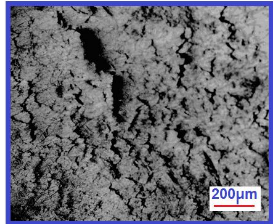
Fig.5. Optical micrograph of stress-ruptured specimen after 11.8h at 1023K and 94.6MPa.
