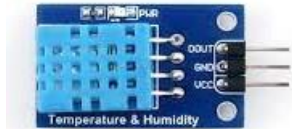
Fig 5: Humidity and temperature Sensor
