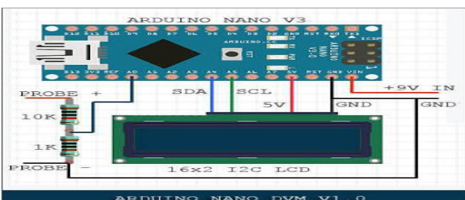
Fig 5. LCD Pin Configuration.
