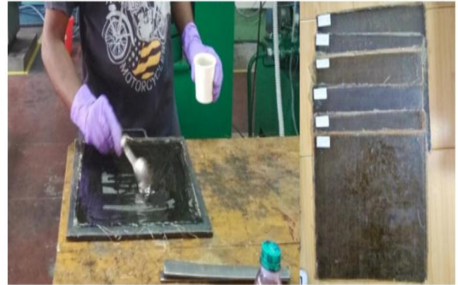
Fig. 3. Hand layup of composites
