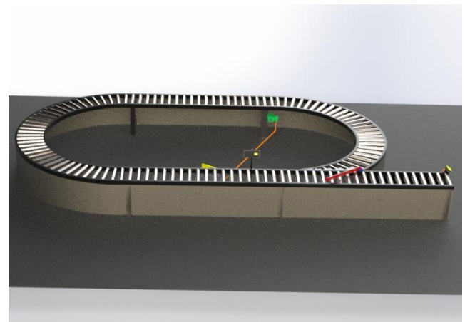
Fig. 4. Image of the belt driven roller conveyor
