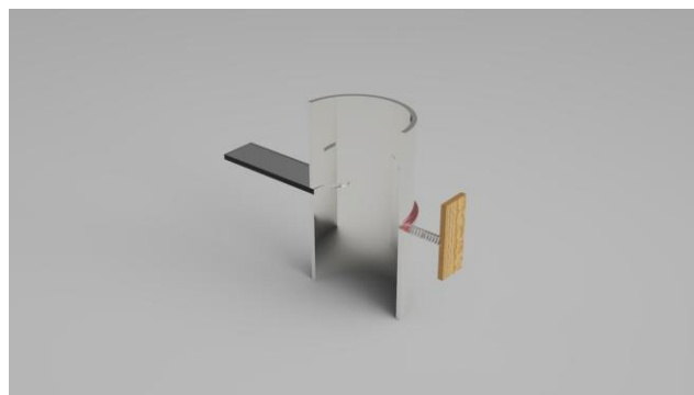
Fig 6. The mechanism used for glass/color filter introduction
