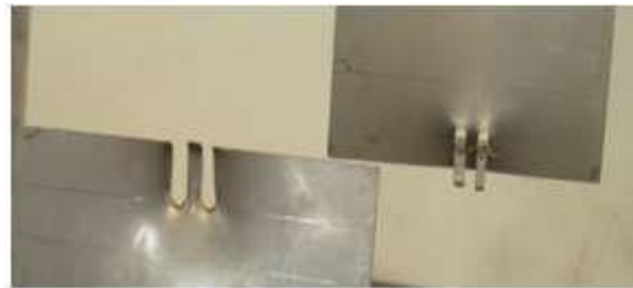
Fig.5 .Pull out failure mode
