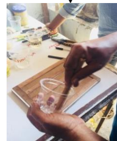
Fig 11: mixing resin and hardener
