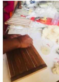
Fig 10: applying PVA coating on mold
