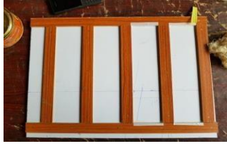
Fig 7: wooden mold to prepare composite material
