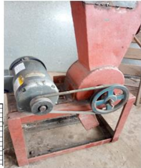
Figure 4: Exploded view of a modified palm nuts cracker Figure 5: The developed centrifugal palm nuts cracker
