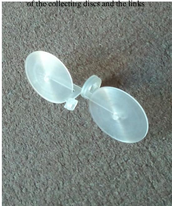
Link with its polypropylene collecting discs
