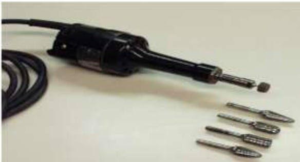
Figure 4: Typical Burr grinder (FHWA, 2013 [6]).
