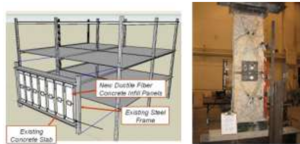
Figure 2. HPFRC infill retrofit system and double infill panel specimen after cyclic testing (Hanson and Billington 2009).
