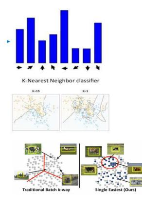
The nearest neighbor classifier simply takes the description of a scene (Bags of SIFT) and calculates the "closest" Euclidean match to the training data. K-NN algorithm is a nonparametric method for classification.
