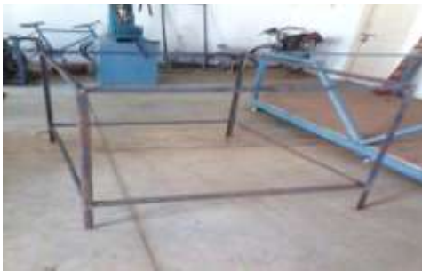
Figure 2.1: Frame of the table (Dimensions of the table: 3×3×4 feet)
