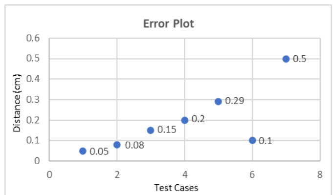
Fig. 10. Error Points of Ultrasonic Sensor
