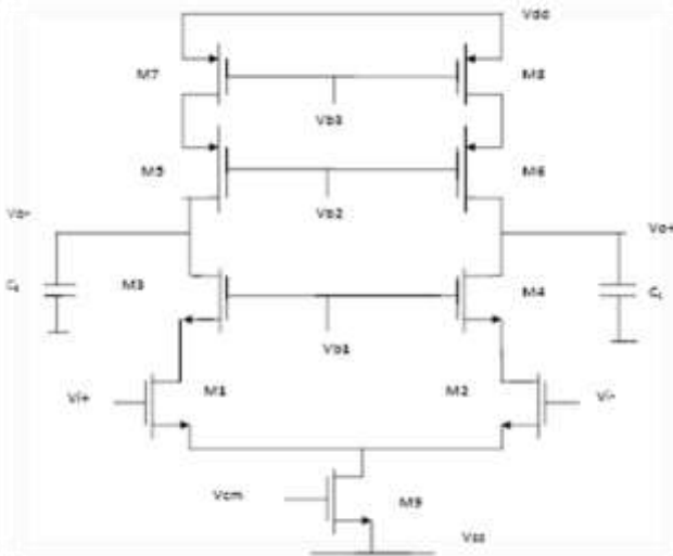
Figure 1.1: Telescopic differential amplifier
