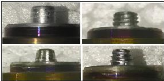
Fig.2 Cylindrical and Conical tools shape
