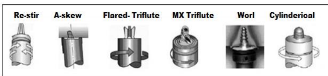
Fig.10 some tools pin of various design.
