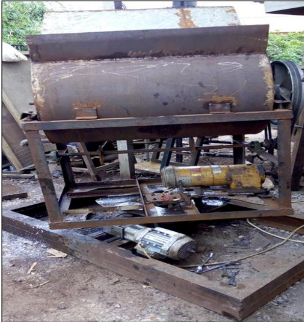
Fig. 5 Fabricated Cassava Peeling Machine
