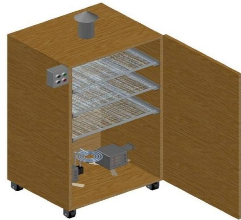
Figure 1 a. Assembled drawing of the vegetable dryer
