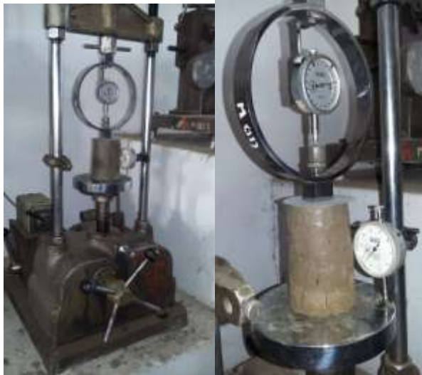
Fig 1. Placement and loading of sample on unconfined compressive strength machine and failure of sample during UCS.
