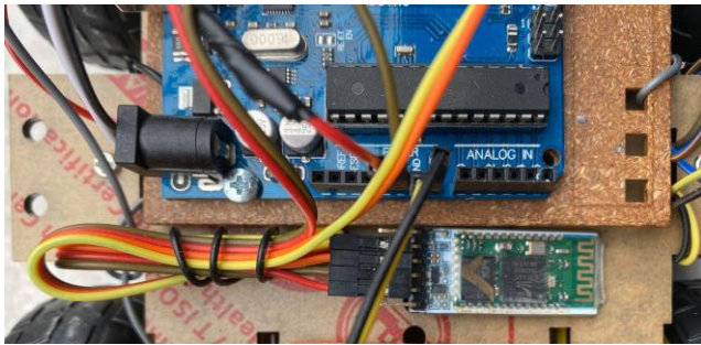
Fig. 3. Bluetooth module mounting and testing.
