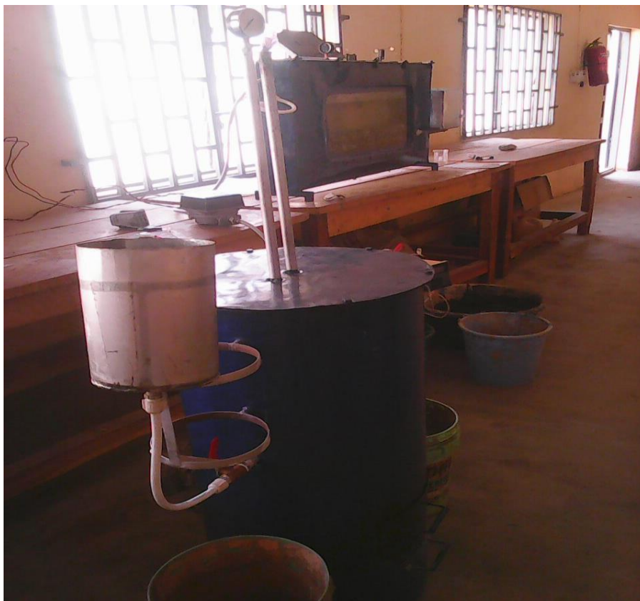
Plate 3: The complete set-up for the remediation of water contaminated with NAPLs consisting of steam boiler, sandbox and the vibration producing electric motor
