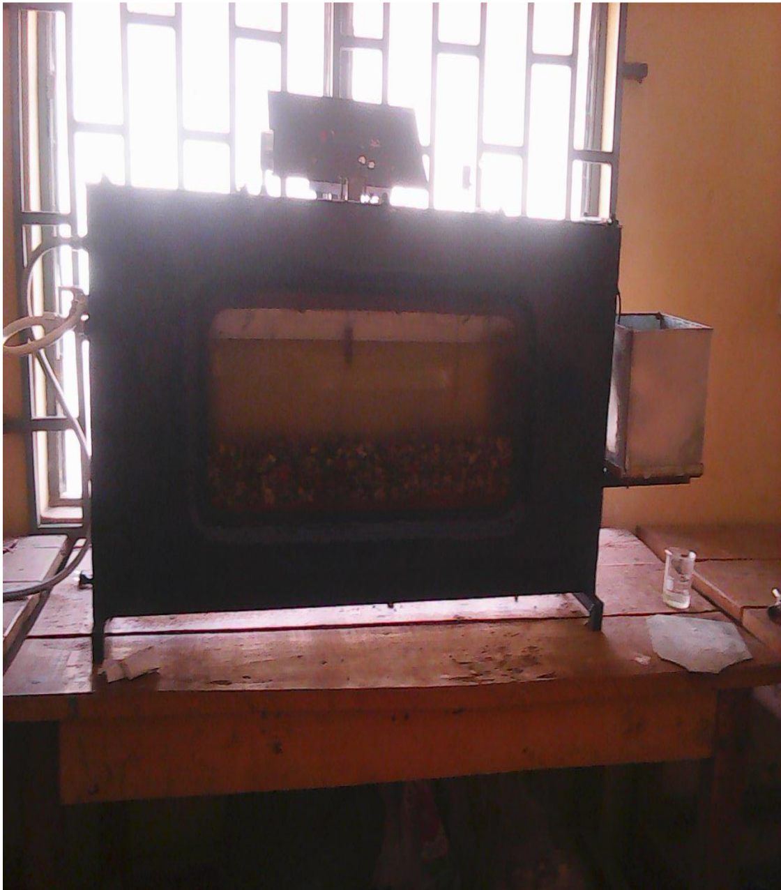
Plate 1: Sandbox containing the ideal soil profile and the mixture of water and the contaminant
